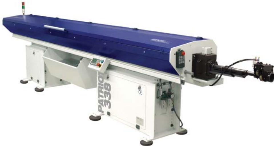
(Caption) The Edge Bar Feeder Patriot 338 is an economically priced 12' magazine bar feeder that features a 3-38mm and diameter capacity, polyurethane guide channels and bushing blocks, hand-held pendant and a 'Swiss Package' including a synchronization device and dual anti-vibration devices.
