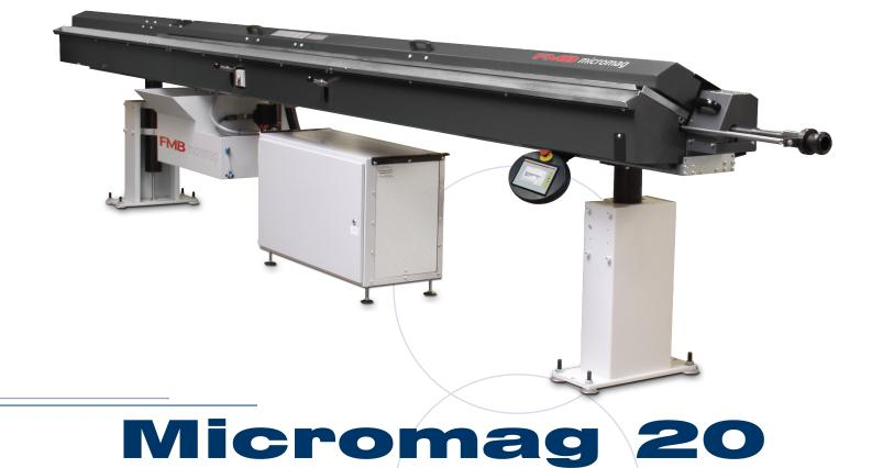
The FMB Micromag 20 is an automatic magazine style Bar Feeder for processing bars in the diameter range of 0.8mm - 20mm in lengths from 12' to 14' on CNC lathes. Equipped with a Swiss type headstock synchronization device, peck drilling and threading on small diameter bars is simple and done with close tolerances. To increase the productivity on your Swiss type lathe, the Micromag 20 is a smart choice.
