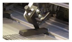
• **Length Monitoring** By inserting maximum and minimum length dimensions into the control, it serves as a safety device, shutting down the magazine if a mis-feed should occur.
