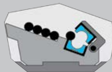
Bar Separation The material is loaded from the bar storage table into the guide channel.
