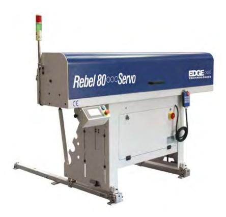
(Caption) Edge Technologies will feature the Rebel 80 Servo at WESTEC 2015. This Rebel is an economically priced servo-driven short bar loader that features an 8-80mm diameter capacity range for automatically feeding round, square and hexagonal bar stock into CNC lathes.
