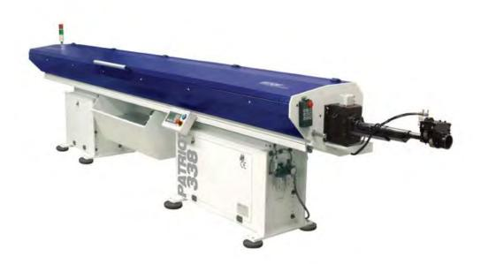
(Caption) The Edge Bar Feeder Patriot 338 is an economically priced 12' magazine bar feeder that features a 3-38mm and diameter capacity, polyurethane guide channels and bushing blocks, hand-held pendant and a 'Swiss Package' including a synchronization device and dual anti-vibration devices.
