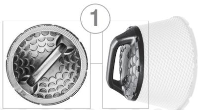
**1st-Stage Separation:** The coolant mist airstream initially collides with the fish scale profile coalescing the mist into larger droplets. Then, through a wind shear effect with the 70-degree, self-draining mesh filter, additional smoke and particles greater than 2 microns ( $2\mu\text{m}$ ) are captured.
