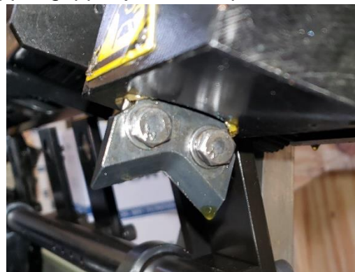
Upper gripper jaw with replacable insert.
