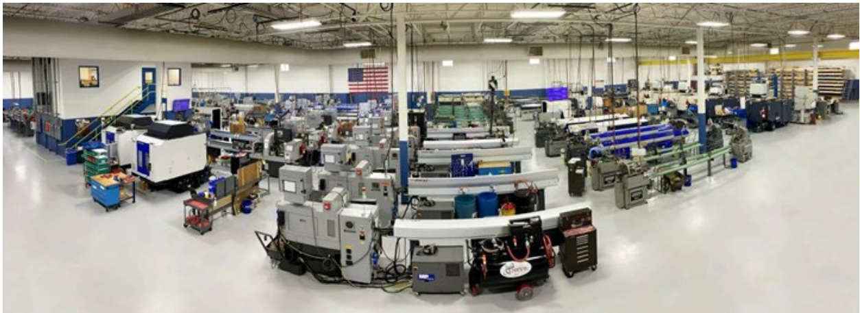
Precision Plus runs 33 CNC Swiss lathes, 9 CNC turn/mill centers, and 30 cam-actuated Swiss lathes.
