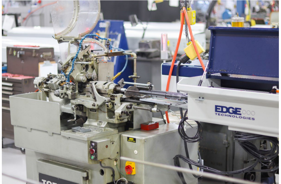
The cam-actuated Swiss lathes have the lowest operating costs and can often yield the best return per square foot.
