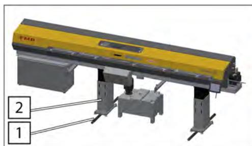
1. → Position the round material bars 1 so that the loading magazine is as close as possible to the lathe.
