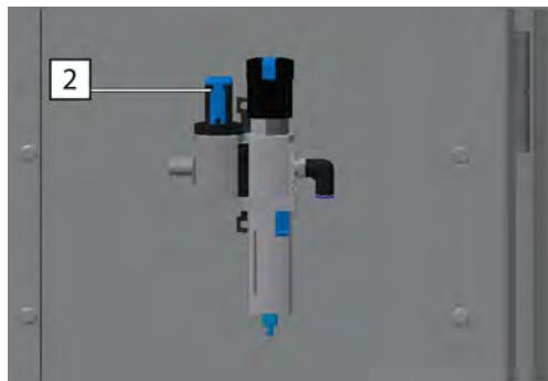
The supply of compressed air is switched on/off at the maintenance unit **1**.
