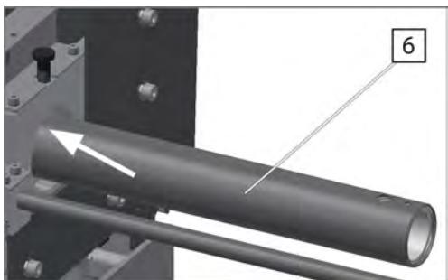
10. Pull the index pin
