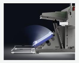
**Folding axial shift.** The folding axial shift allows for easy maintenance and spindle liner changes. The shifting device is standard in X-axis, optional with Z-axis.
